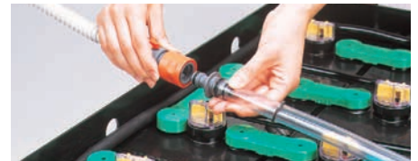
Refilling preparation: Snap-connect the couplings of the hoses on the tank and battery sides and open the faucet.
